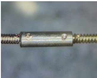
Welding of end faces of nickel-titanium spring wires
