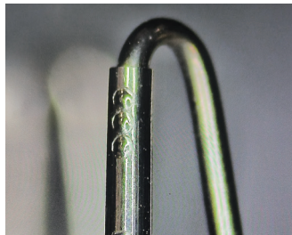
Welding of metal wires through sleeves
